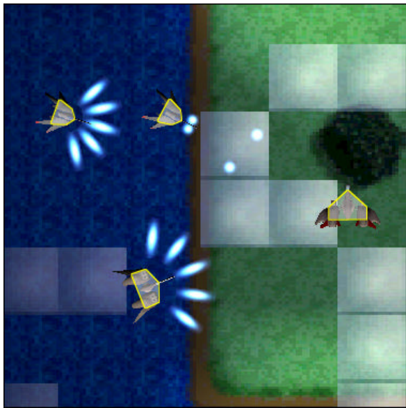
Figure 9: Ship-Ship collision detection using polygonal armatures in a game engine. Image taken from the Broadsword project, copyright © A. Phelps and A. Cloutier, Rochester Institute of Technology 2003.
